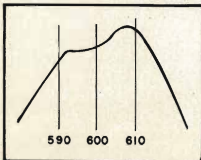
Figures 3a, b, c and d (below). In a appears an ideal bandpass characteristic. In b we have a narrower pass band. The sidebands corresponding to 10-kc modulation would not be heard when receiver is exactly tuned to the carrier. In c and d appear tuning effects when one or more single-tuned resonant circuits are used.
